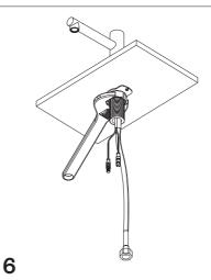
Slide the backnut over the flexible hose and sensor leads. Tighten using
