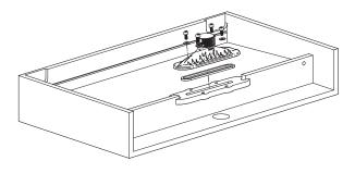
Ensure that the sealing gasket is correctly fitted into the recess on the funnel and tighten the 4 bolts.
