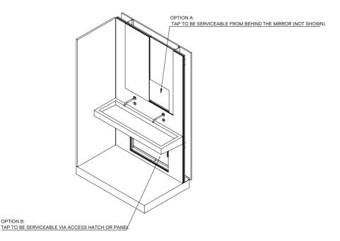
Ensure access hatches below the washbasin and/or behind the mirror are accounted for to ensure easy access of components during installation and for routine maintenance.
