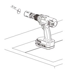
Drill hole 7/8" diameter in wall 8-10" above the bottom of the basin.
