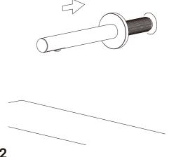
Fit dispenser body into the 7/8" hole in wall.
