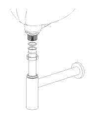
Place flat washer within the notched nut, and screw onto basin waste thread. The washer should be between the adjustable inlet tube and the basin waste.
