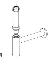
Push the adjustable tube into the main body to a height of your preference. Once set at the right height, screw the plain nut tight onto the main body of waste trap.
