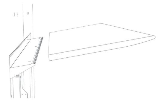
STEP 16 - Install the washplane (Part A) by carefully sliding into the reveal.
