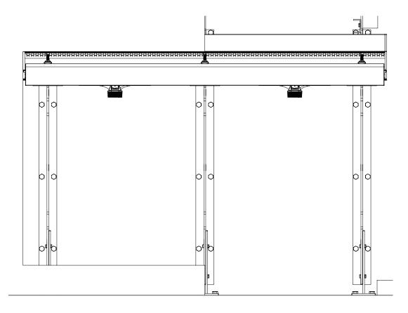
STEP 15 – Board your wall making sure to leave aperatures for access, above and below the aerofoil system.
