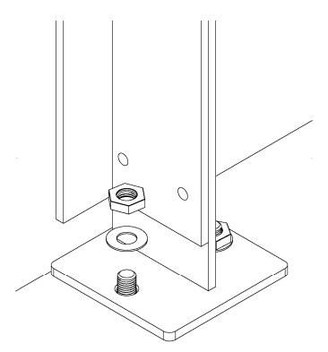
STEP 6 – Secure the support frame to the floor. Depending on your floor build-up, the type of fixing used will vary. The illustration shows anchor fixings which would be suitable for concrete floor slabs. (Fixings not included.)
