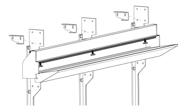
STEP 13 - Building up your wall framing using suitable metal or timber walling
