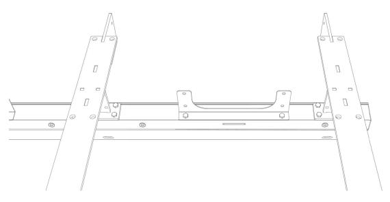
STEP 4 – Position the support frame into its install location. Adjust the height setting using a socket wrench.
