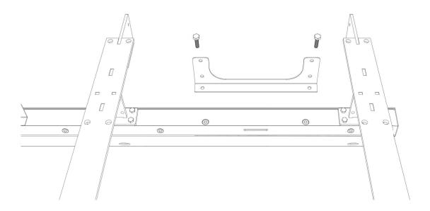
STEP 3 – Position waste support bracket(s) (Part F) and secure to the assembly using a socket wrench
