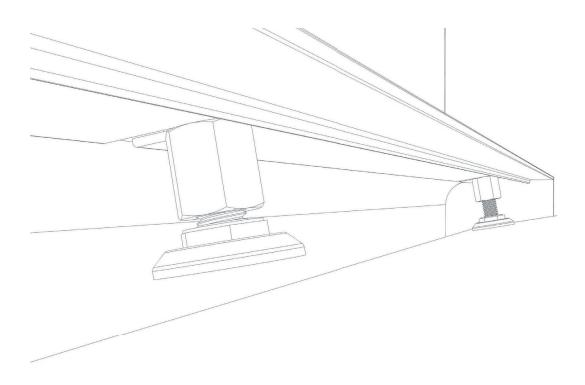
STEP 17 - Secure the leg assembly clamping nuts (Part H) to the washplane (Part A) by tightening with an adjustable spanner.
