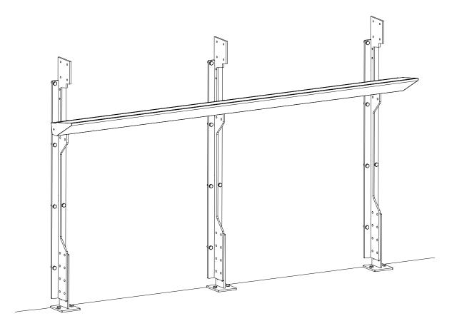
STEP 5 - Ensure the frame is level and mark holes potions.
