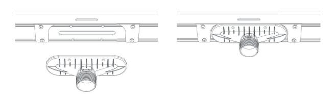
STEP 10 - Fit waste funnel(s) (Part G) using the fixing provided.
