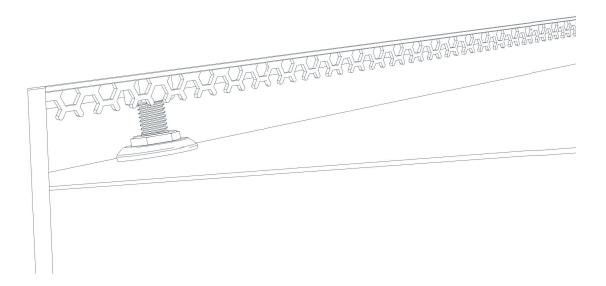
STEP 18 - Lower the grates (Part E) to meet the washplane (Part A)
