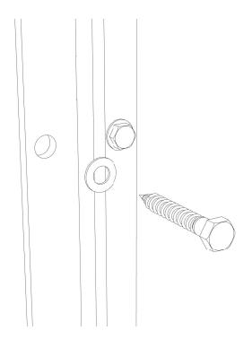
STEP 7- Secure legs to the back wall using suitable washers and fixings
