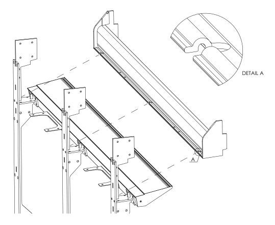
STEP 8 – Lift and position PVC gully extrusion (Part C) onto the assembly. The rear slots will interface with the frame if positioned correctly.
