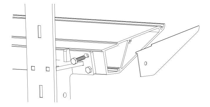
STEP 2 – Using the fixings supplied and a socket wrench, secure parts as shown and clip on the end caps. (End caps are stored inside the washplane extrusion)
