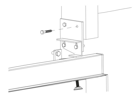
STEP 14 – Fixing holes are provided at the top of each support leg. The type of fixing will depending on your walling system
