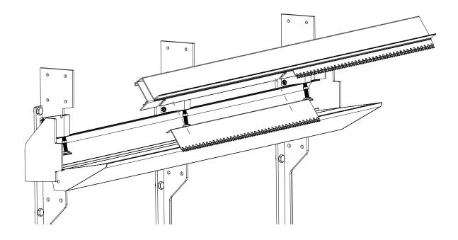
STEP 12 – Insert the grate(s) (Part E) into the grate housing extrusion (Part D). Then lift and position the extrusion (D) onto the assembly. The rear slots will interface with the frame if positioned correctly.
