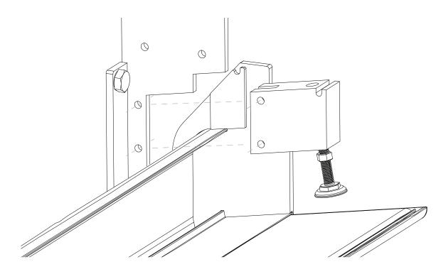
STEP 11 – Refit the clamping blocks to the leg assembly (Part H) as shown and secure using the fixing provided. Secure blocks loosely enough to allow for the grates to be fitted in the next step.
