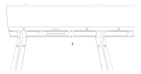
STEP 9 - Secure PVC gulley extrusion (Part C) and waste support bracket (Part F) using the self tapping fixings provided. Ensure the gulley is aligned correctly to the leg assemply before attaching the waste support plate.
