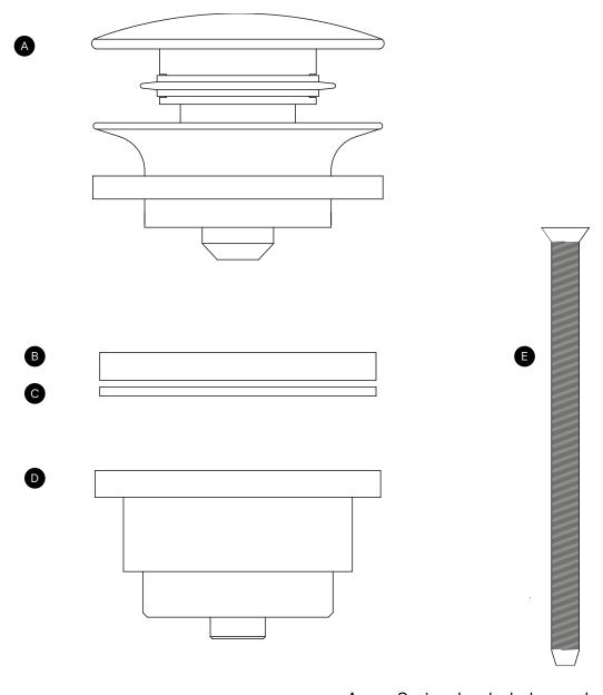
A Spring-loaded plug and waste grate
