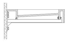
Lift Monolith over the front of the mounting tabs onto the wall brackets
