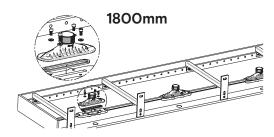
Ensure that the sealing gasket is correctly fitted into the recess on the funnel and tighten the 4 fixing
