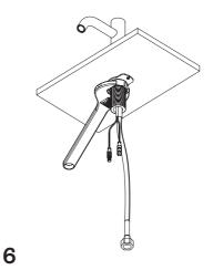
Slide the backnut over the flexible hose and sensor leads. Tighten using a spanner.
