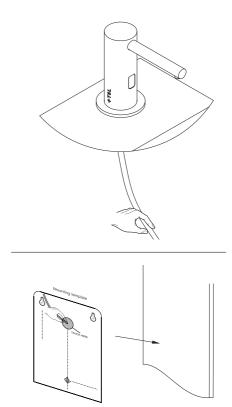
Touch the Mounting template to find the best position for installing.
