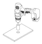
Mark soap hole centres onto the surface Drill 25mm diameter hole in countertop. for installation.
